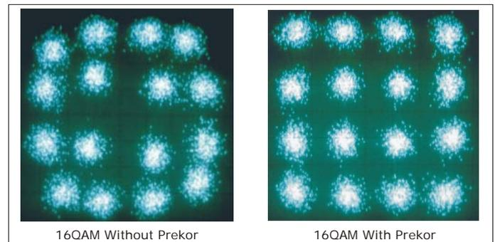
By combining PREKOR and DVB-S2 modulation with MPEG-4AVC compression technology, the satellite distribution can be made highly efficient enabling more services per transponder than any other open system available today.
