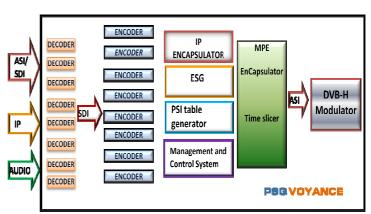
The Voyance mobile TV headend supports simultaneously up to eight independent digital video input (SDI), and MPEG transport streams over ASI or IP inputs and up to 24 embedded AES/EBU digital audio in SDI input. The IP Encapsulator of the unit accepts MPEG 4 video signal from the encoders and converts it into an IP stream. It manages different data types including a single program transport stream and embedded SDI audio streams.
