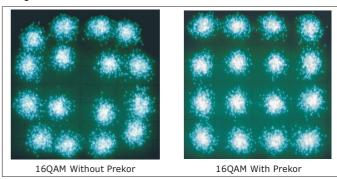
By combining PREKOR and DVB-S2 modulation with MPEG-4 AVC compression technology, the satellite distribution can be made highly efficient enabling more services per transponder than any other open system available today.
